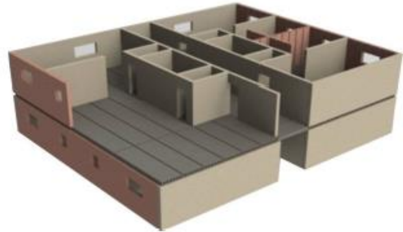
Illustration of load bearing wall structure (fib 74)
